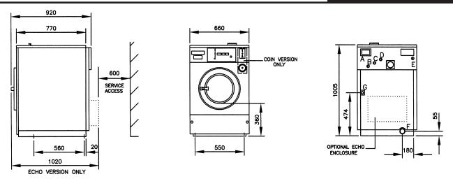
A - Ventilation Overflow Outlet, B - Soft Water Connection (cold), C - Warm Water Connection, D - Hard Water Connection (cold),
